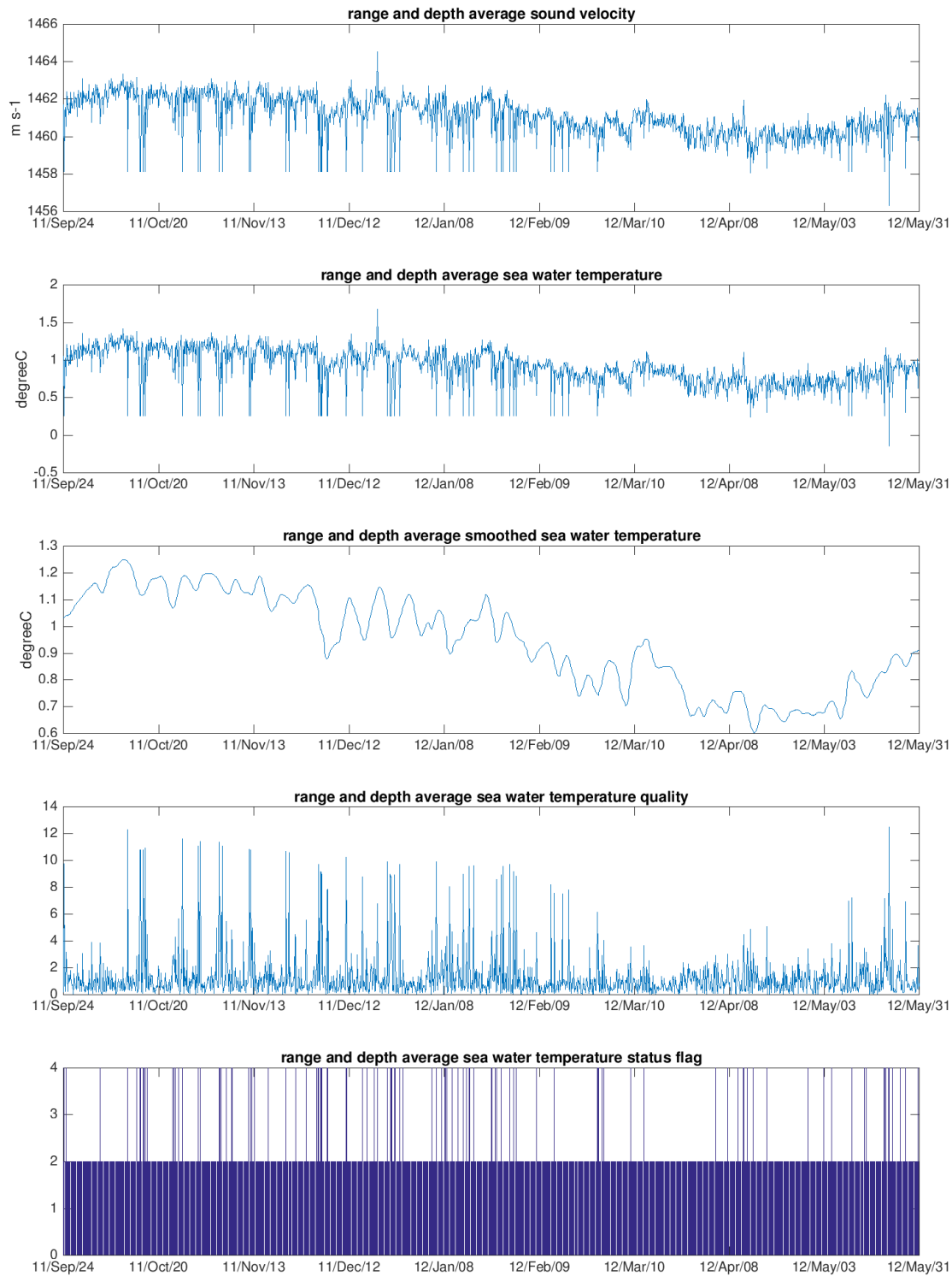
Figure 12-6. Data from ARCTIC_ACOBAR_B-A_20110924-20120531_WSSP_WTMP. nc. The panels are range-depth averaged sound speed in ocean waters ( mean_c ), depth-range averaged ocean water temperature ( mean_t ), smoothed values of mean_t ( mean_t_smooth ) and quality of mean_t ( mean_t_qlty ) from the top respectively.
