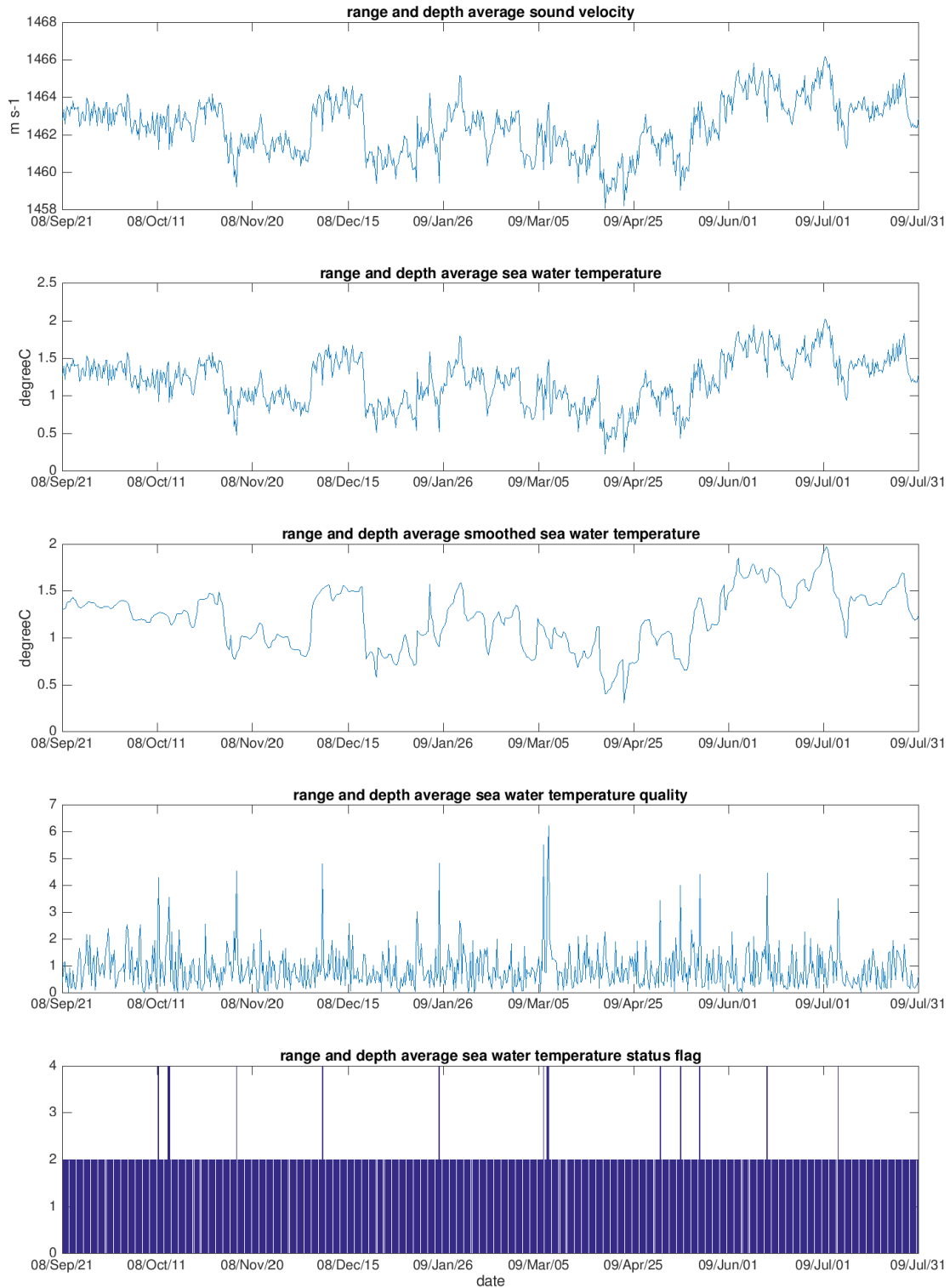
Figure 7. Examples of five variables in the WSSP_WTMP dataset, ARCTIC_DAMOCLES_S-R_20080921-20090731_WSSP_WTMP.nc. The panels are time-series range-depth averaged sound speed in ocean waters ( mean_c ), time-series depth-range averaged ocean water temperature ( mean_t ), smoothed values of mean_t ( mean_t_smooth ) and quality of mean_t ( mean_t_qlty ) from the top respectively.
