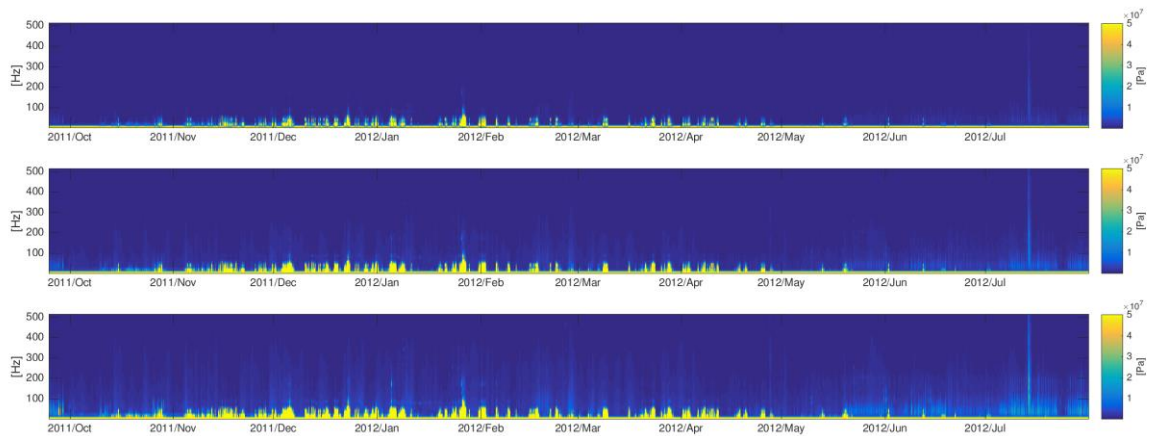
Figure 9. Sound pressure in Pa ( snd_pressure ) from hydrophone-1, in ARCTIC_ACOBAR_A2012_20110924-20120731_ambientnoiseL2 dataset. From the top panel, 10-, 50- and 90- percentiles respectively. The horizontal axis ( time ) is common for all parameters.
