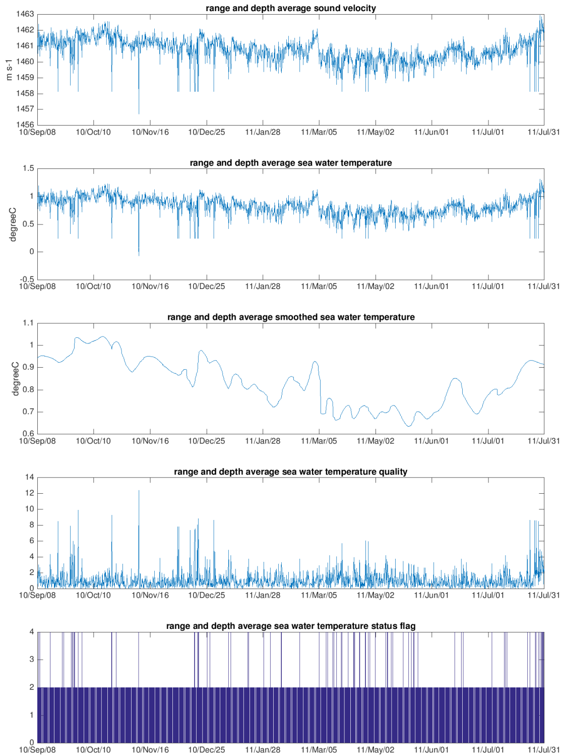
Figure 12-5. Data from ARCTIC_ACOBAR_B-A_20100908-20110731_WSSP_WTMP. nc. The panels are range-depth averaged sound speed in ocean waters ( mean_c ), depth-range averaged ocean water temperature ( mean_t ), smoothed values of mean_t ( mean_t_smooth ) and quality of mean_t ( mean_t_qly ) from the top respectively.
