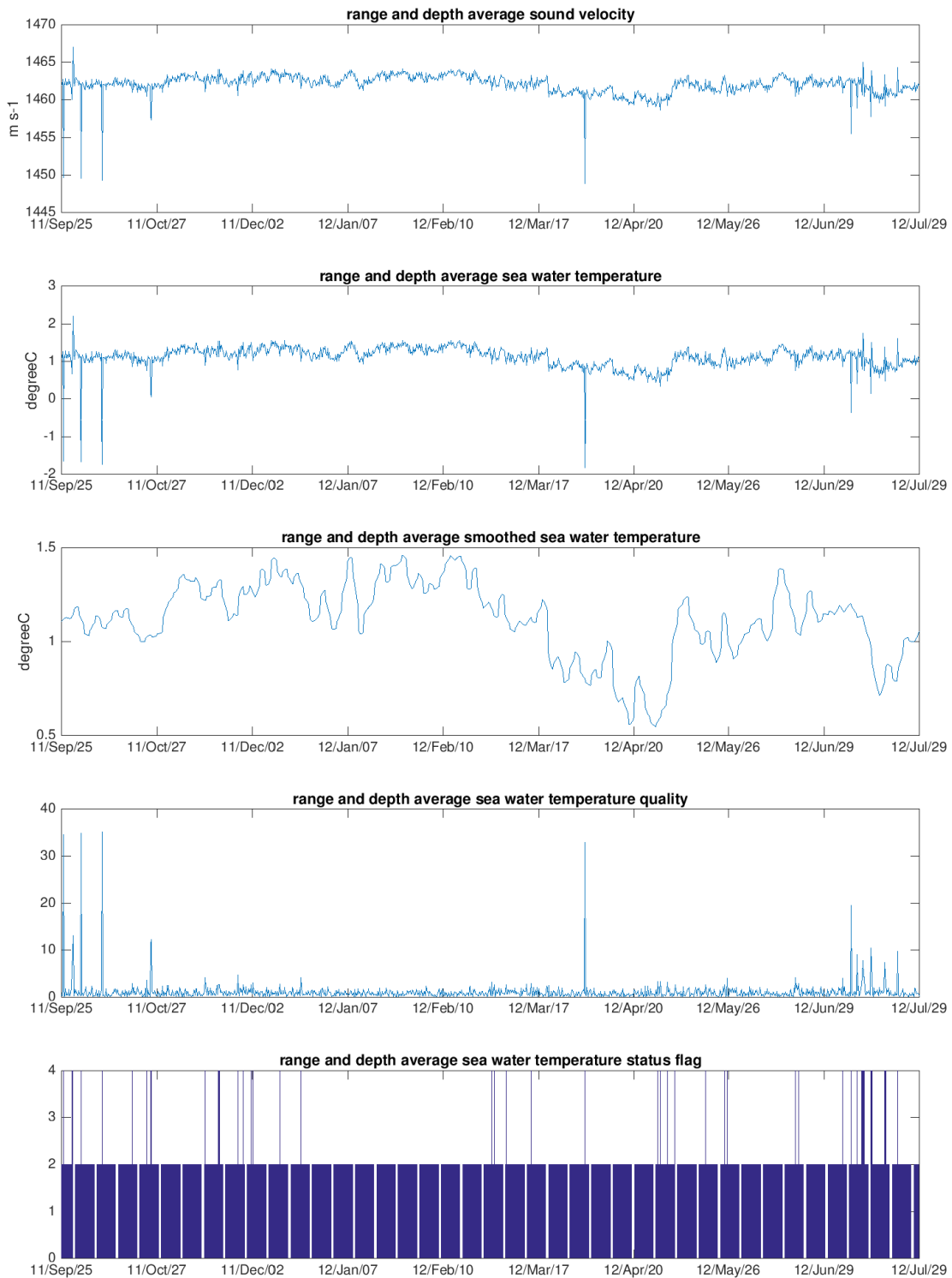
Figure 12-4. Data from ARCTIC_ACOBAR_A-D_20110925-20120729_WSSP_WTMP.nc. The panels are range-depth averaged sound speed in ocean waters ( mean_c ), depth-range averaged ocean water temperature ( mean_t ), smoothed values of mean_t ( mean_t_smooth ) and quality of mean_t ( mean_t_qlty ) from the top respectively.
